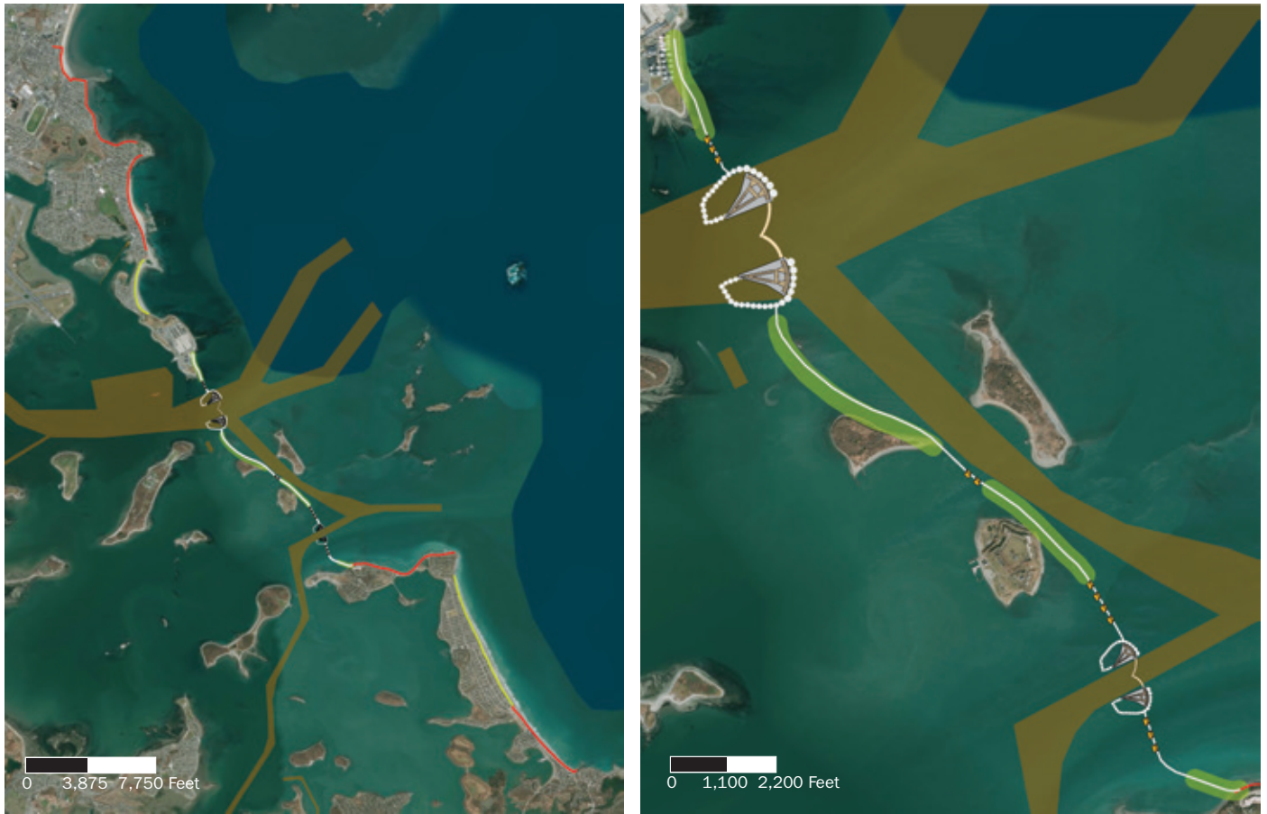
FIGURE 4.5 Outer Harbor Barrier Configuration
