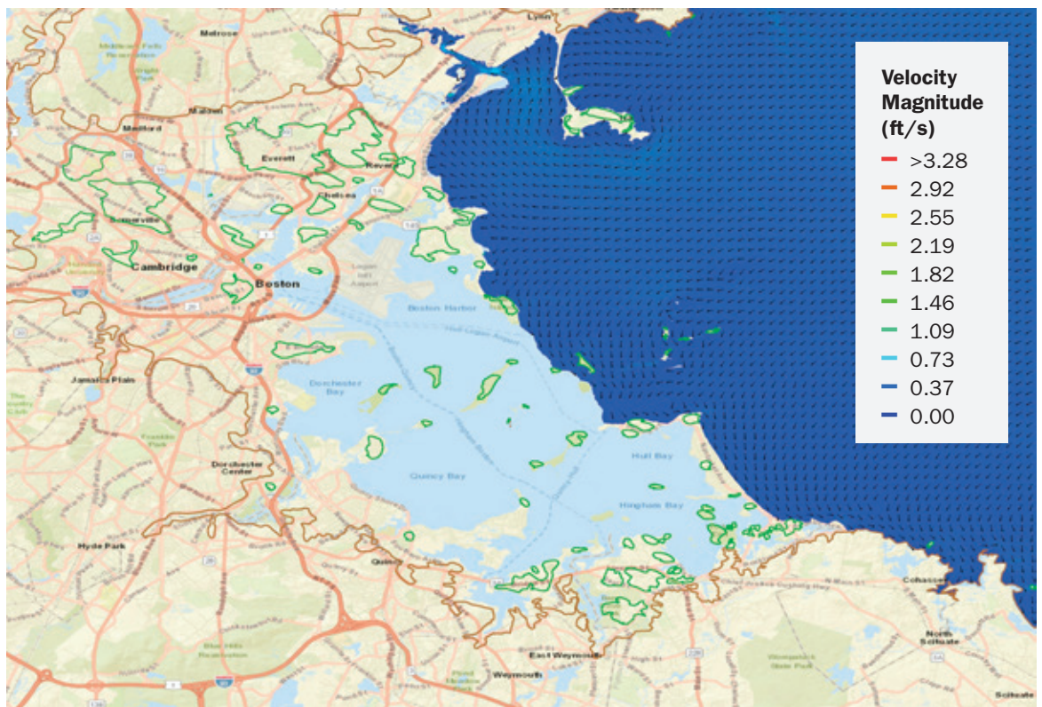
FIGURE 5.15 Circulation with Barrier Closed During Storm
