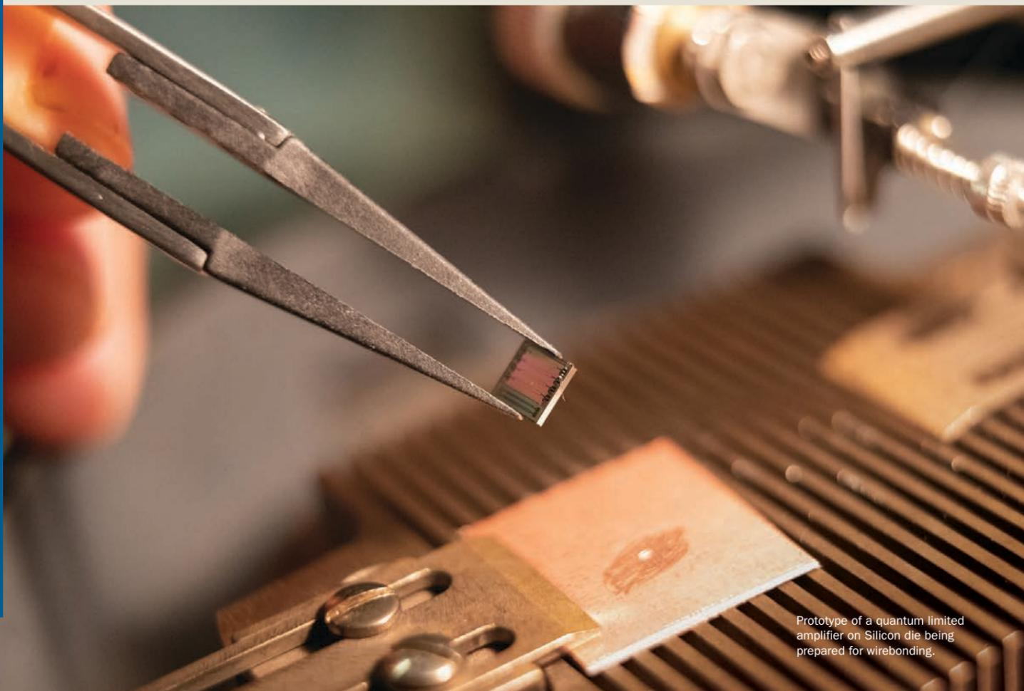
Prototype of a quantum limited amplifier on Silicon die being prepared for wirebonding.
