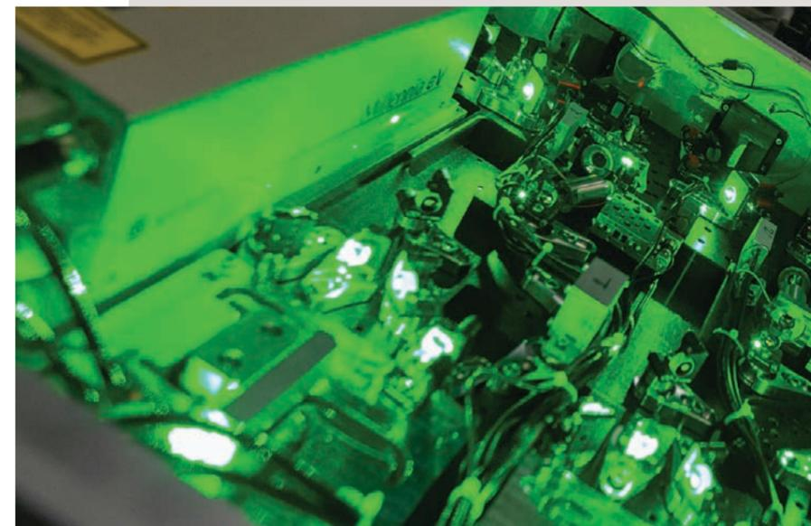
▲ Ultra-short pulse, mode locked laser system used for laser spectroscopy to characterize and investigate quantum system.
