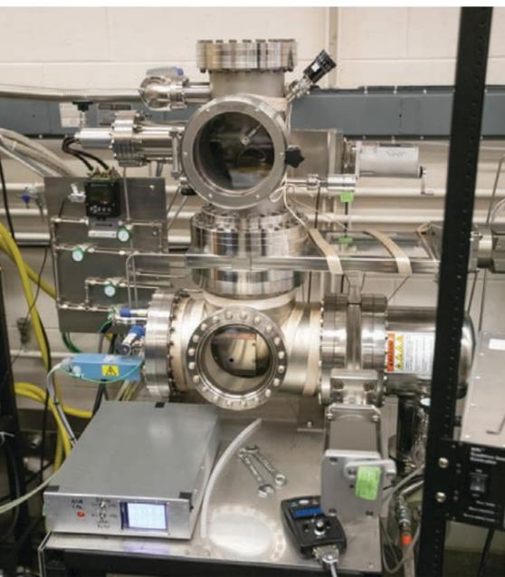
▲ Ultra-high vacuum deposition system used for quantum circuit fabrication.
