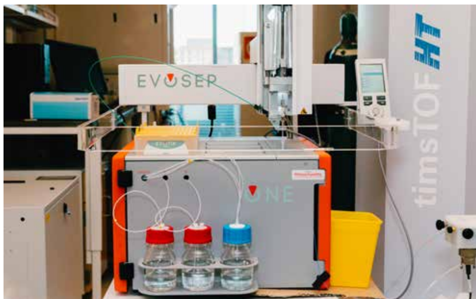
The EvoSep nanoHPLC that is used in conjunction with our timsTOF.
